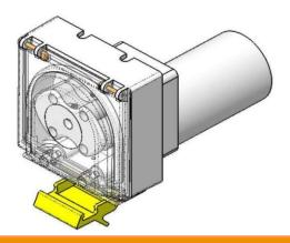
The 4000 is a high performance and versatile peristaltic pump. The hinged lid forms an integral part of the pump construction, and releasing the lid catch facilitates tubing replacement. The lid can also be removed completely for tube replacement in confined spaces.
